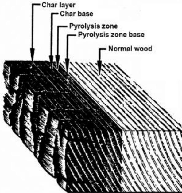
What does this illustration tell us about fire behavior? The first is that wood exposed to high temperatures will decompose. When it does decompose, it provides an insulating layer of char that retards the further degradation of the wood for period of time. This means that the fuel side of the tetrahedron is a variable that is always changing when a fire is in progress.
